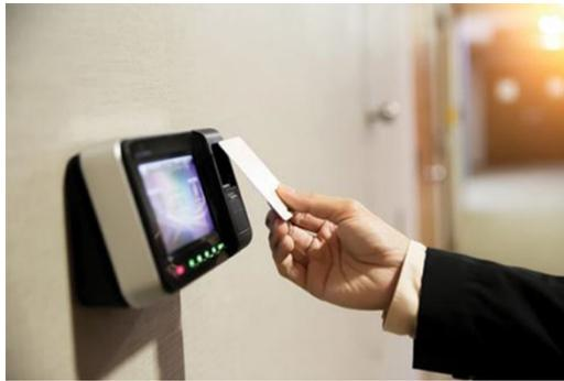
**Gambar 3.14:** Radio Frequency Identification Device (Noah, 2020)
