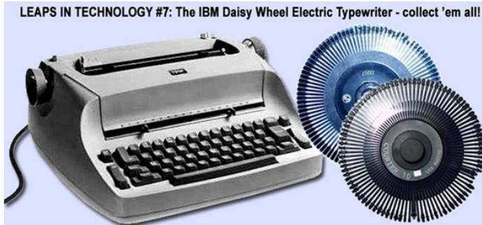
**Gambar 4. 7:** Daisy wheel printer (Joyprintsolution, 2018)
